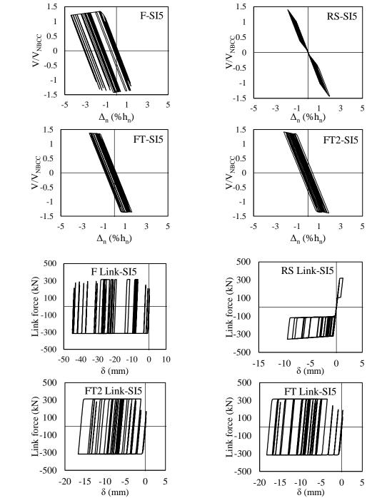
*Figure 7. a).* Storey shear vs storey drift hysteretic responses of the systems *b).* Load vs. deformation response of the friction dampers (links) of the systems
