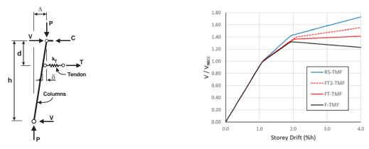
Figure 3. Equilibrium of the FT-TMF system upon activation of the dampers. Figure 4. Load-deformation responses of the TMF systems studied
