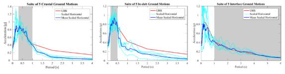
Figure 5. 5% damped spectra of the ground motion records of each suite.
