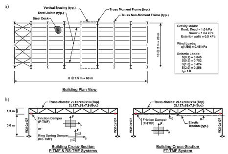
Figure 2. Building studied: a) Building plan view and design loads; b) Building cross-sections illustrating the F-TMF, RS-TMF and FT-TMF systems.
